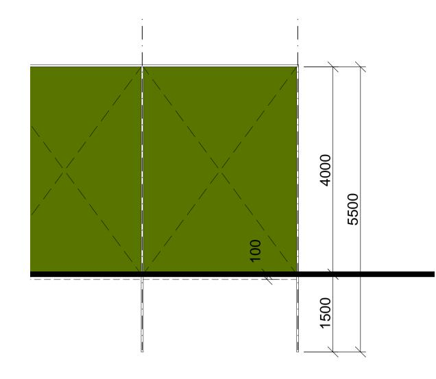
PROPOSED ACOUSTIC FENCING DETAIL 1:50 @A1
