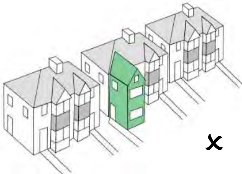
An unacceptable front extension
